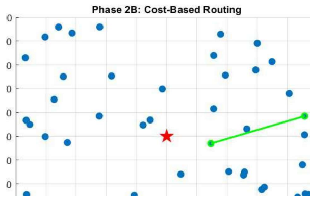
Fig. 3. Phase 2B: Cost-Based Routing – path selected using distance and link quality cost.
