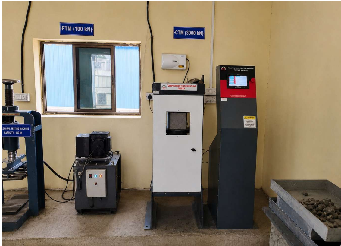
Figure 1 Experimental setup for compressive strength testing.
