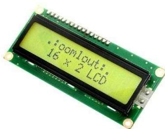
A 16×2 LCD (Liquid Crystal Display) is one of the most commonly used display modules in embedded systems and Arduino projects. It can display 16 characters per line and has 2 lines, hence
