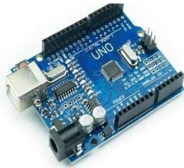
The Arduino Uno is one of the most popular microcontroller boards used for electronics projects and embedded systems. It is based on the ATmega328P microcontroller.
