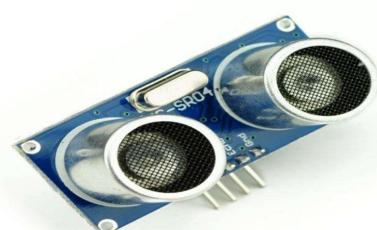
The HC-SR04 Ultrasonic Sensor is a popular distance measuring sensor that works on the principle of sound wave reflection. It measures the distance between the sensor and an object by sending ultrasonic waves and calculating the time taken for the echo to return.
